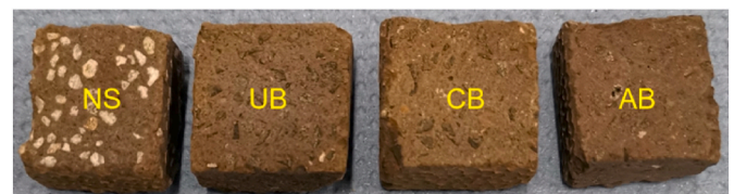
Fig. 2. Cubic mortar pieces for SEM analysis.
