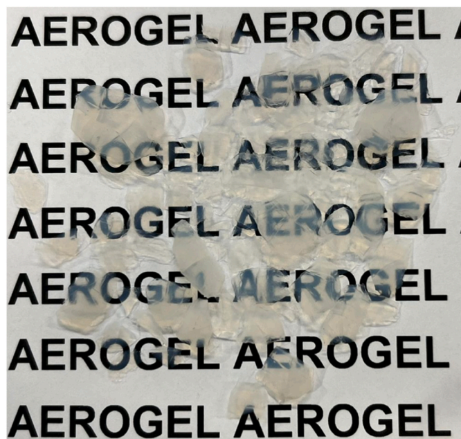
Fig. 2. Photo of silica aerogel particles prepared from waste glass.
