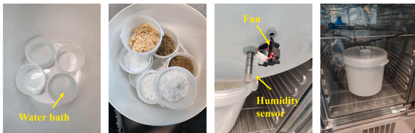
Fig. 3. Experimental setup of water vapour sorption test; (a) water bath at the bottom; (b) samples above the water bath; (c) humidity sensor and a fan setup; (d) climate chamber.
