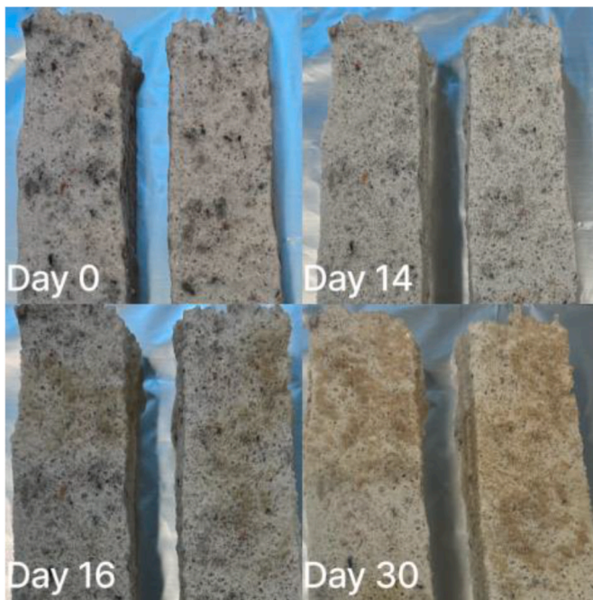
Fig. 20. Wet samples in conditioning climate chamber – Reference.
