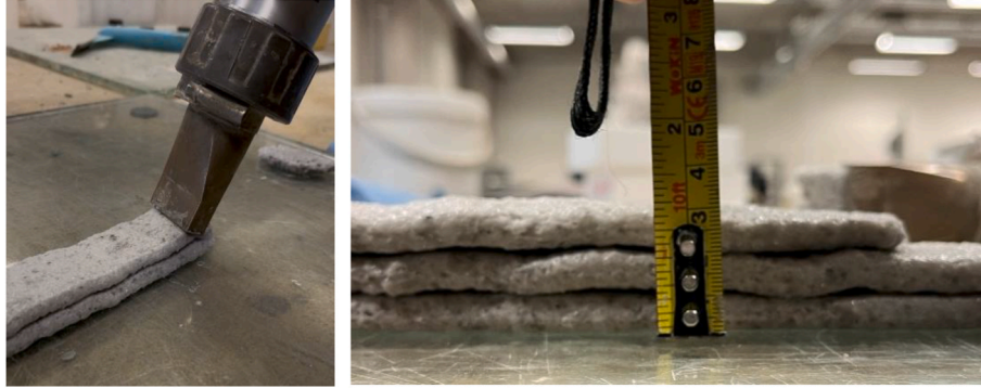
Fig. 7. Hand-free printing of insulation material.
