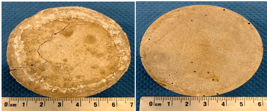
Fig. 12. Observation of top (left) and bottom (right) view of puck render.
