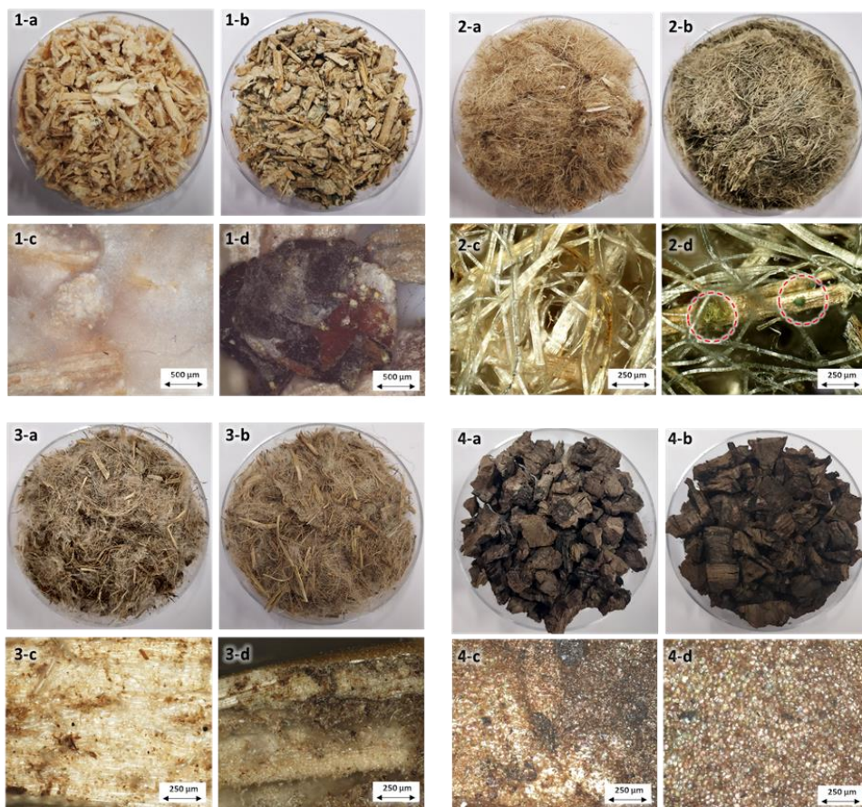
Fig. 2.10 Mould evaluation test (1) mycelium, (2) hemp, (3) grass and (4) cork composites. For the subset, (a) and (c) are samples without conditioning, (b) and (d) are samples conditioned under high RH.
